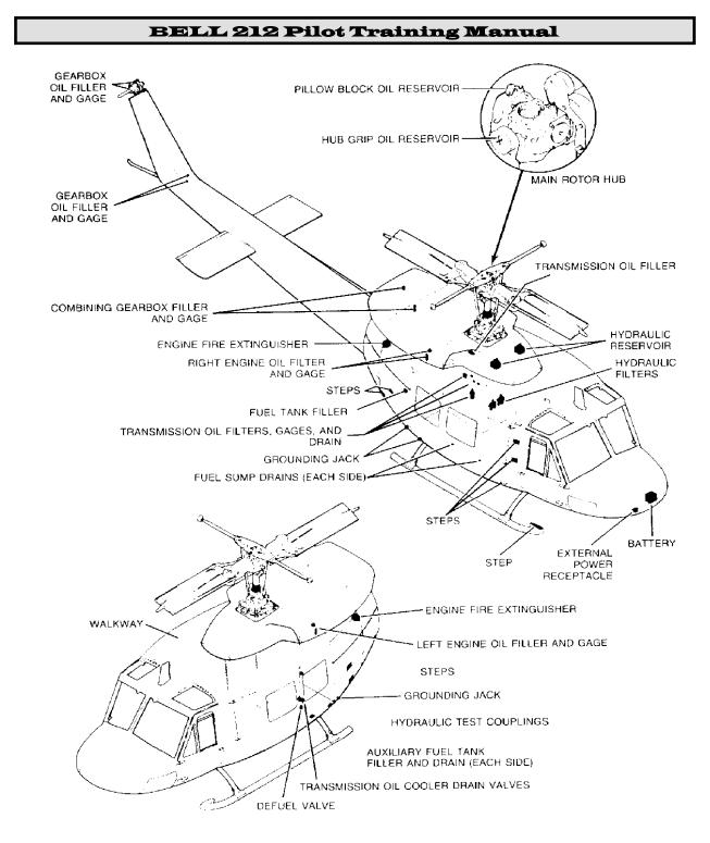
Figure 2-20 Inspection and Servicing (Sheet 1 of 2)
