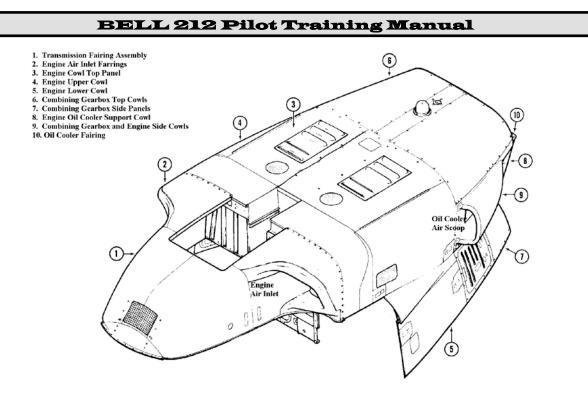
Figure 2-15 Transmissions and Engine Cowling
