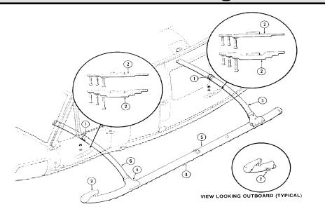
Figure 2-16 Skid Landing Gear
