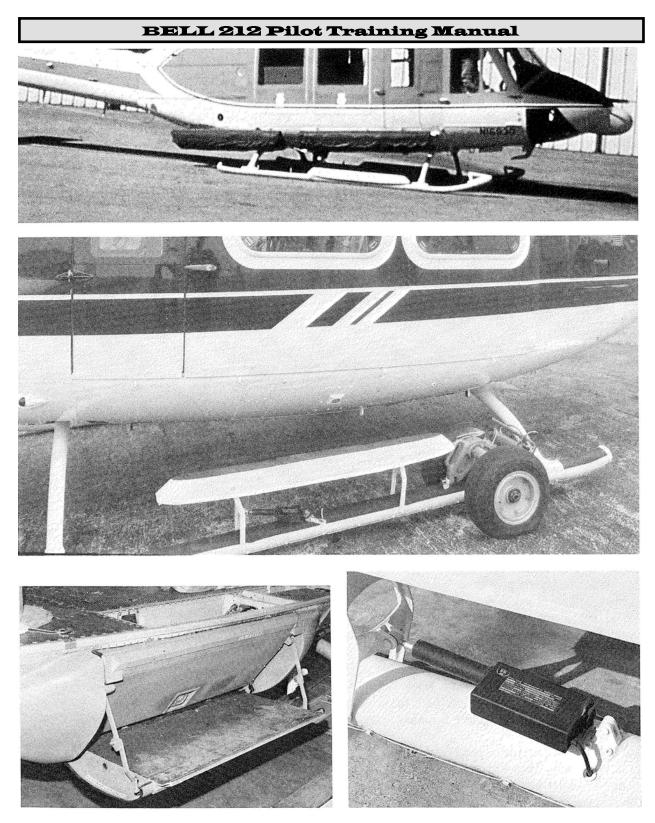
Figure 2-17b Passenger Step Kit Variants in Use with Floats
