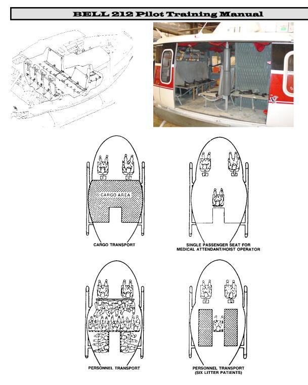
Figure 2-5Seating Arrangements(At Campbell normally only Cargo and Personnel arrangements)
